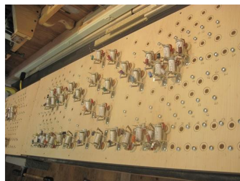
The magnets & pallets wired to the underside of the topboard of the chest to cover the air holes when the pipe is not playing
