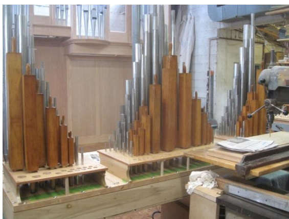
The positif division chest that feeds air to the pipes
